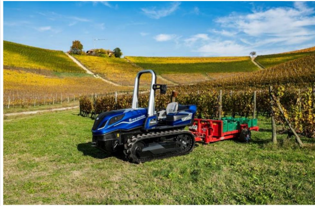
FIGURE 5 Prototype of crawler endowed with F28 gas engine in practice field test.
